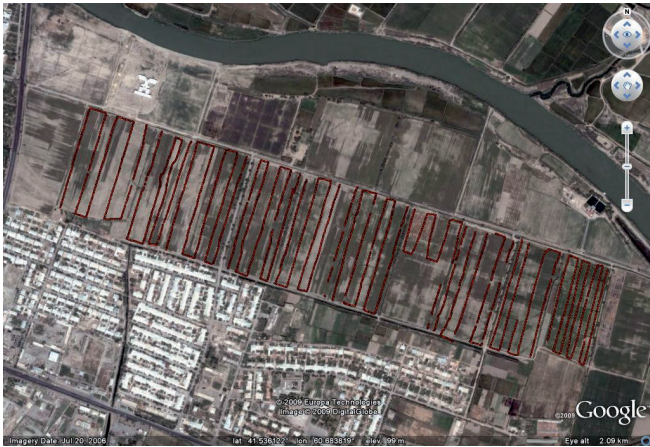
Picture 2: Illustration of measurements conducted using EM38 in a pilot area of around 70 hectares
