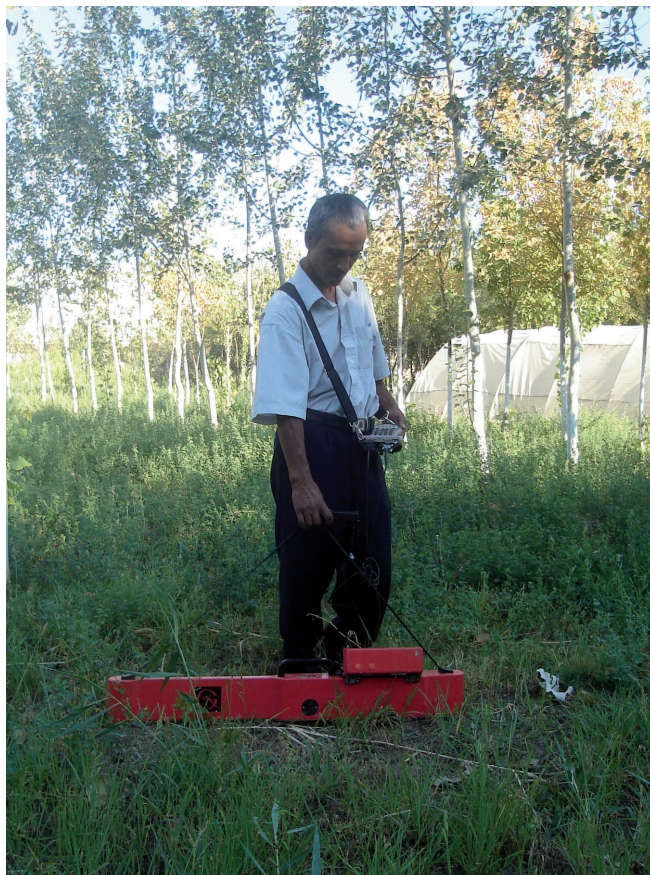
Picture 3: The use of EM38 in the field by operator
