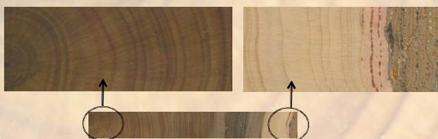
Fig. 4 Scanned J. procera disk sanded with 600-grit sandpaper and scanned with 600 dpi scanner.
