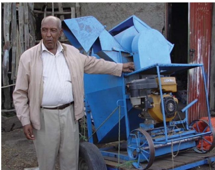
Ethiopian farmer Adebabay with one of his four thresher units which have improved the quality of tef
