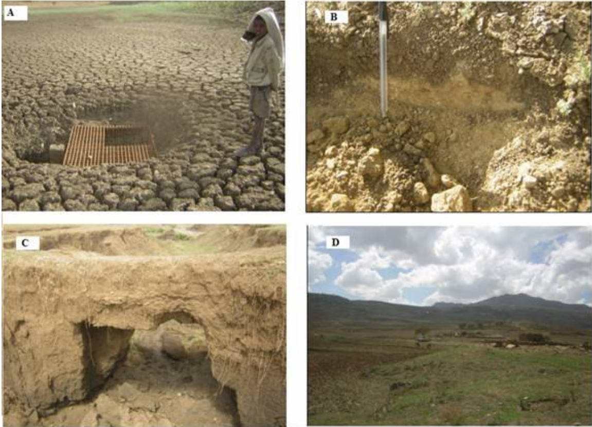
Figure 2: Selected characteristics of reservoirs/watersheds:(a)-silt deposit overtopping the inlet box at Grashito, (b)- difference in soil colour and level of consolidation to identify the sediment depth (at the periphery of Grashito reservoir, (c)- deep gully incision with in Filiglig watershed which extends up to the grazing land (see Figure 3), (d)- part of the Filiglig watershed peripheries which are bare with few scattered trees
