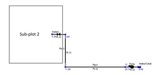
The system delivers to the sub-plot 2 a Flow rate of 76.32 m<sup>3</sup>/hour with a Pressure of 5.25 m.w.c and a flow velocity of 1.24 m/s (figure 7).
