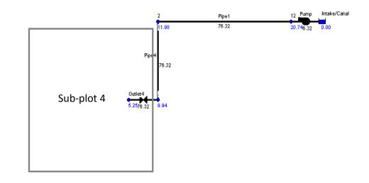
The system delivers to the sub-plot 2 a Flow rate of 76.32 m<sup>3</sup>/hour with a Pressure of 5.25 m.w.c and a flow velocity of 1.24 m/s (figure 9)
