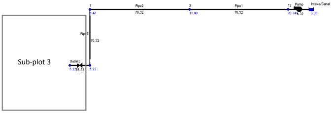
The system delivers to the sub-plot 3 a Flow rate of 76.32 m<sup>3</sup>/hour with a Pressure of 5.22 m.w.c and a velocity of 1.25 m/s (figure 8)
