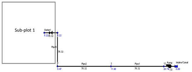
The system delivers to the sub-plot 1 a Flow rate of 76.32 m<sup>3</sup>/hour with a Pressure of 5.22 m.w.c and a flow velocity of 1.24 m/s (figure 6).
