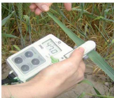
SPAD measurement in winter wheat at heading stage
